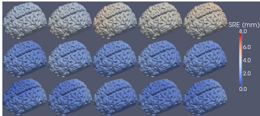
Fig. 7. SRE computed for each point in the surface model for the five tracked pointer (top row), five LRS (middle row), and five conoprobe (bottom row) datasets of the brain phantom. Registration error increases from blue to white to red.
